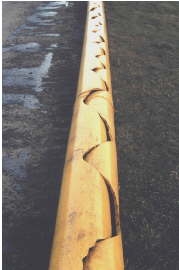
Figure H.1 RCP in 315 mm SDR 17.6 PE80 pipe
